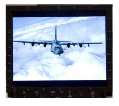
The GECO SXGA Multi-Function Display supports conversion of interlaced analog video in NTSC and STANAG A (525 lines) or STANAG C (875 lines) to digital video for output to a high quality 1280 x 1024 17-inch LCD TFT display. The video source is selectable from a primary
